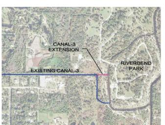
Canal 3 Extension in Jupiter Farms reduces headloss and provides better stormwater runoff management for the area
